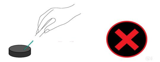
Longitudinal Hall probe: When the magnetic field line enters the Hall sensor from the sensing end of the probe, the DSG-510 reading shows a symbol of+or N, and vice versa, the symbol is - or S
