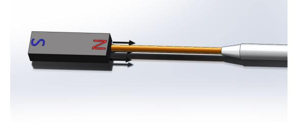
Schematic diagram of longitudinal Hall probe testing solenoid magnetic field: Place the longitudinal probe in the central area of the solenoid and perpendicular to the magnetic field line
