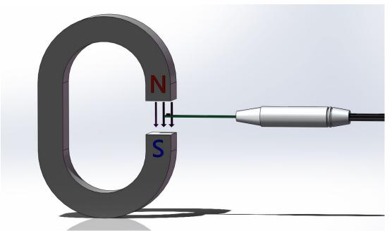
Place the convex side of the probe (i.e. the side with the chip sealing side) horizontally on the surface of the tested magnet or the magnetic field measurement point to measure the surface magnetism of the magnet.
