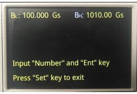
B<sub>L</sub>: lower limit set value: when it is displayed in white, it can be modified by number keys, and the upper and lower limit input status can be switched by Ent key. When the test data is lower than the lower limit set value, press Ent key in the test display Home screen to display NG unqualified, and the display time is about 3 seconds.
